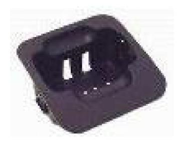
Icom AD-100 charger adaptor for BC-119N & BC-121N for IC-M87.
