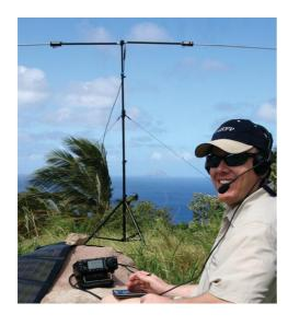
The buddipole portable antenna dipole kit 40-2m 250w.
